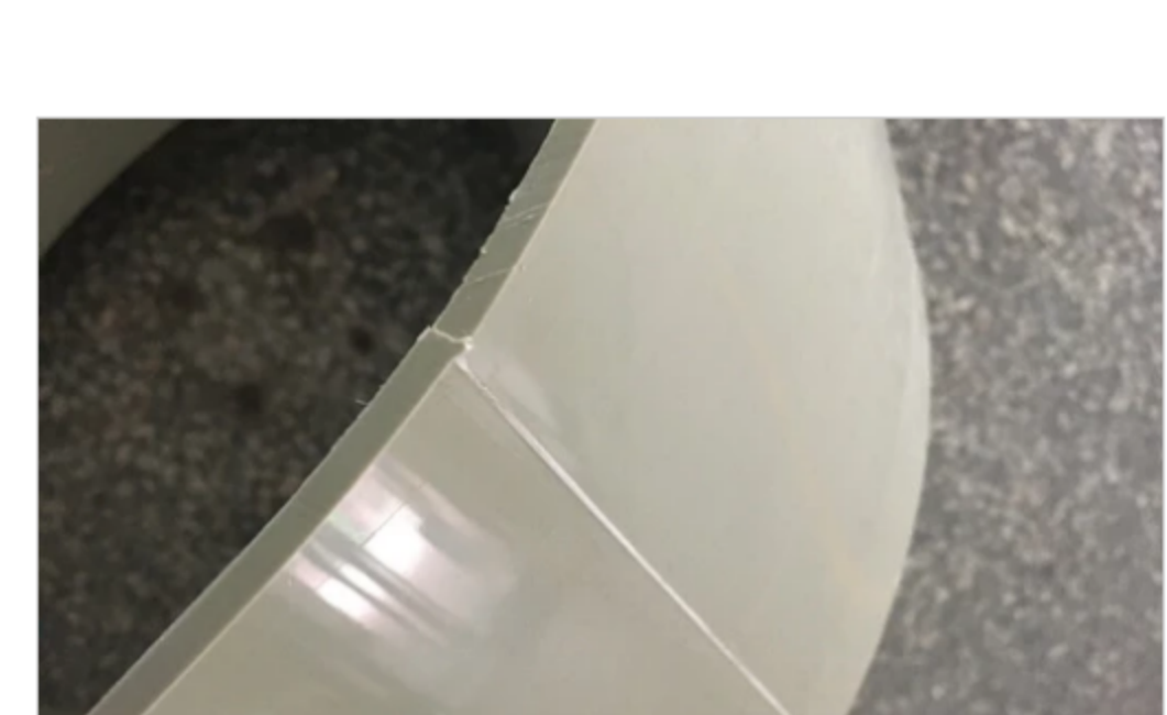
Butt welding HDPE board to a circle
