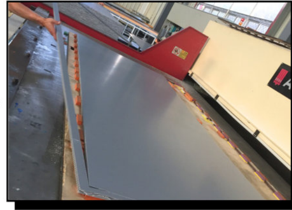
c. Die Cutting: High-precision die cutting ensures the pallet sleeve is shaped accurately to fit the container design.
