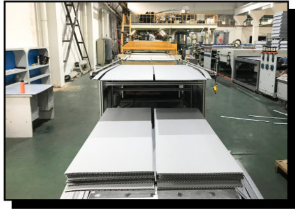
a. Board Production: The pallet sleeve is made from lightweight PP honeycomb panels by extrusion technology for durability and impact resistance.
