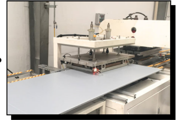
d. Creating Door Openings: Small windows are cut into the sleeve, allowing quick access to the contents without fully opening the container.
